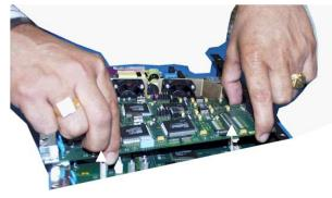
now empty slot is to remain unused, be sure to install a 6KPM-BLNK face plate cover.
